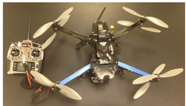
Note: The images acquired from the GoPro camera in flight were geo-tagged and processed for the orthomosaic image and point cloud data in 3D coordinate system to represent surface features.
