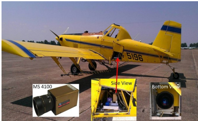
Figure 1 MS 4100 camera-based multispectral imaging system on the Air Tractor 402B behind with data-communication Magma PCI box and rugged laptop hosting navigation software
